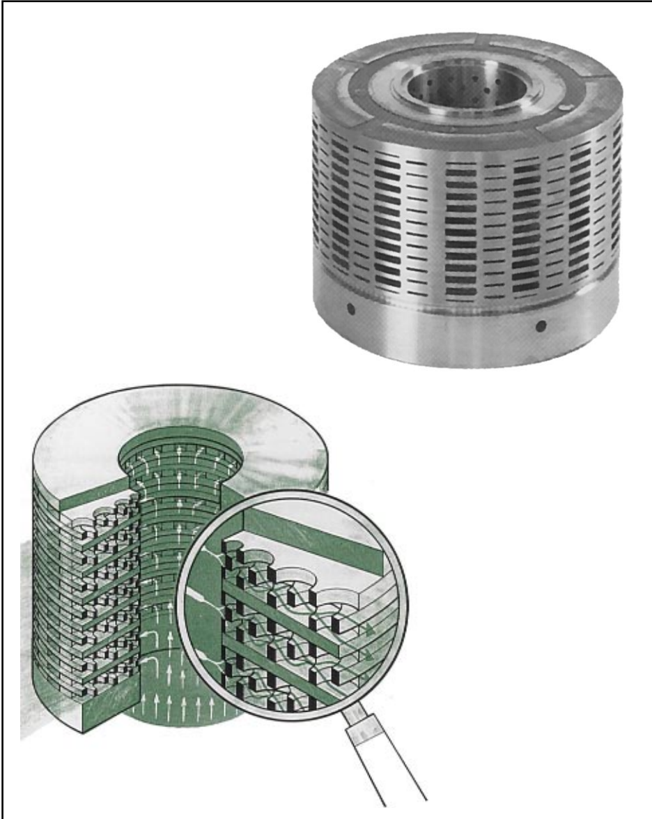
Fig. 12 Trim of LIMIPHON control valves of universal multistage/multipath type, provided with labyrinth disk stack. Fluid paths are obtained by overposing disks suitably drilled and mutually oriented.
