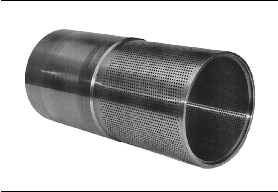
Fig. 10 GBR type single cage - The noise reduction is obtained by providing a very high number of low diameter holes (2÷4 mm) Acoustic attenuation up to 15 dB.
